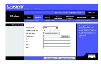
Figure 8-26: Wireless Tab - Wireless Security (WEP)
